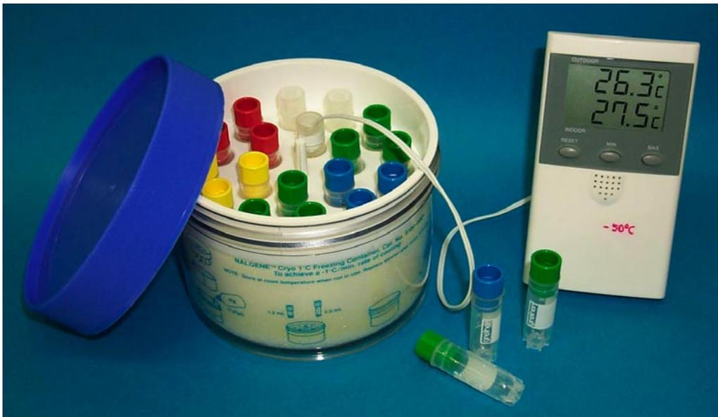
**Figure 16.** Slow freezing using Nalgene™ cryo 1°C Freezing Container with temperature probe.
