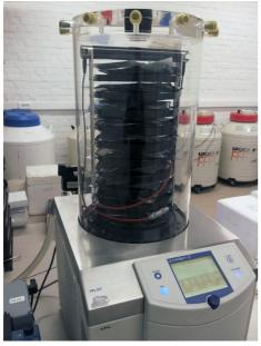
Freeze-drying device for leaf samples
